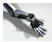
touch, pressure, humidity and temperature placed in the fingers which makes them even more complicated. Each finger has 4 degrees of freedom grouped in 3 joints by means of which their mobility is identical to the one of human fingers.
